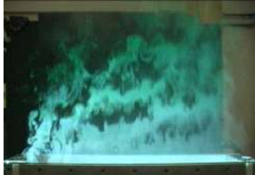
Views output chimney (hot) in the median plane for \Delta T=10^\circ \text{C}
